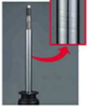
Damage on surface of piston rod as in photo.
